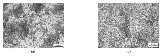
Fig.1. Undesirable microstructure after spheroidization (a) lamellar pearlite (b) residual pearlite.
