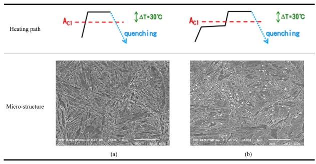
Fig.5. Microstructure after quenched by performing different heating paths.<sup>(2)</sup>
