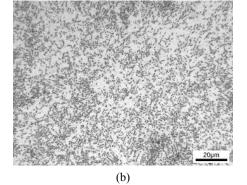
Fig.8. The microstructure acquired from different spheroidized annealing pattern (a) Pattern A (b) Pattern B.
