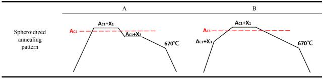
Fig.7. Spheroidized annealing patterns.
