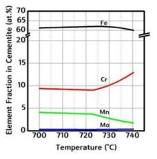
**Fig.4.** Element fraction in cementite changed with temperature by using the JMatPro® simulation.<sup>(2)</sup>
