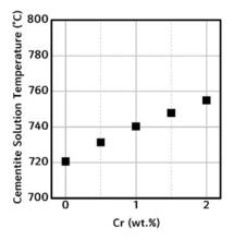
**Fig.3.** Cementite solution temperature varied with Cr content by using the JMatPro® simulation.<sup>(2)</sup>
