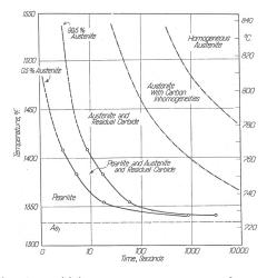
**Fig.2.** Austenitizing rate temperature curves for commercial simple-carbon eutectoid steel.<sup>(4)</sup>
